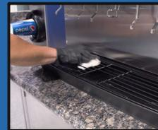
Clean the drain pan and drip tray with unscented disinfecting wipes
