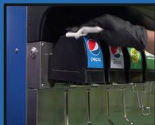
Wipe down the external surfaces of the valve covers & actuating levers with unscented disinfectant wipes
