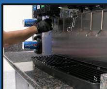
Replace the nozzles and diffusers back into the bottom of the valves
