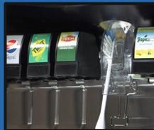
Immerse a clean brush in sanitizing solution & clean the entire ice chute. Allow to air dry
