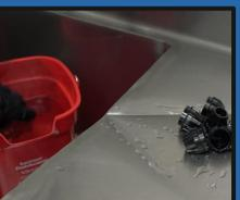
Place nozzles and diffusers in sanitizing solution for 60-90 seconds. Remove and allow to air dry on a clean surface
