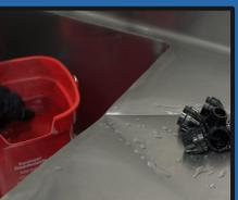
Place nozzles and diffusers in sanitizing solution for 60-90 seconds. Remove and allow to air dry on a clean surface
