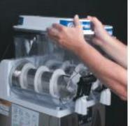
and remove the hopper lid(s). lift slightly. NOTE: On Autofill models, remove the level probe and fill tubes from the hopper.
