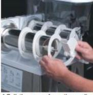
1. Unplug the hopper lamp cord(s) 2. Depress the hopper lock plunger, 3. Pull the hopper assembly forward 4. Pull the auger from the cooling 5. Remove the hopper seal from the drum.
