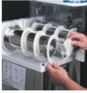
augers. Push the augers as far as and cooling drum and slide it into with lamp cord at the back. they will go and rotate them so the place. Push down until the hopper flat face of the auger shaft is aligned lock plunger snaps into place. with the flat face of the auger nose. NOTE: On Autofill models, install
