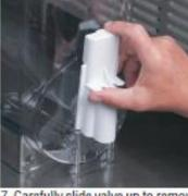
spring and faucet seal. Extra care from inside the front of the hopper. seal to prevent damage.
